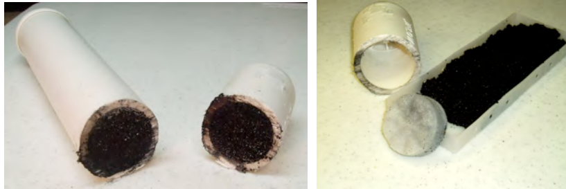
Cutaway view of a replacement refrigerator 'filter' cartridge and its carbon contents
