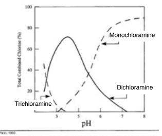
Figure 6-2. Distribution Diagram for Chloramine Species with pH
