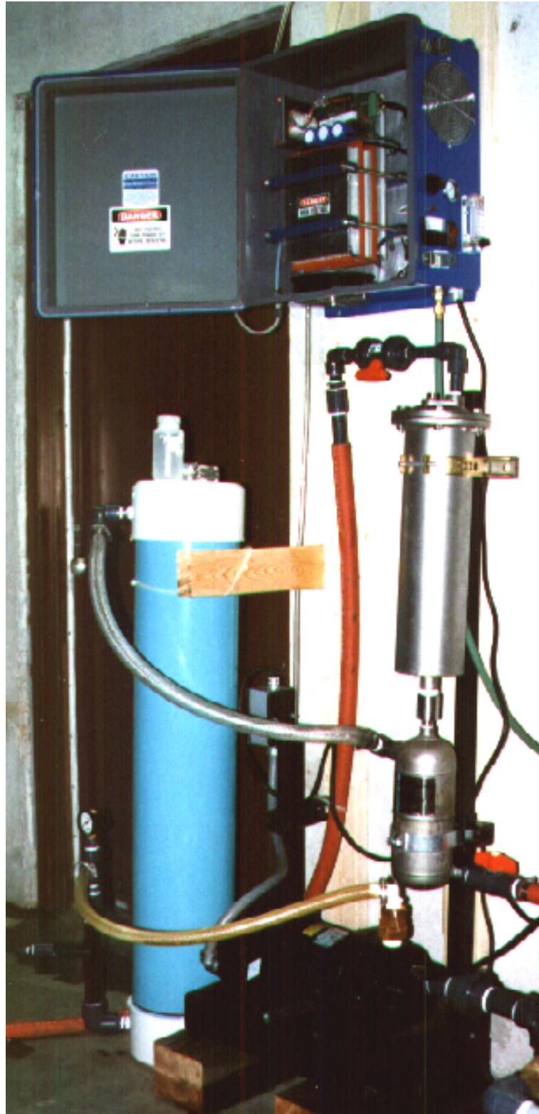
Ozonation System: Flat-Plate Ozone Generator, Venturi Injector (Mazzei), Contacting Tank (WMU, blue column) and Degassing Separator (GDT, stainless steel)
