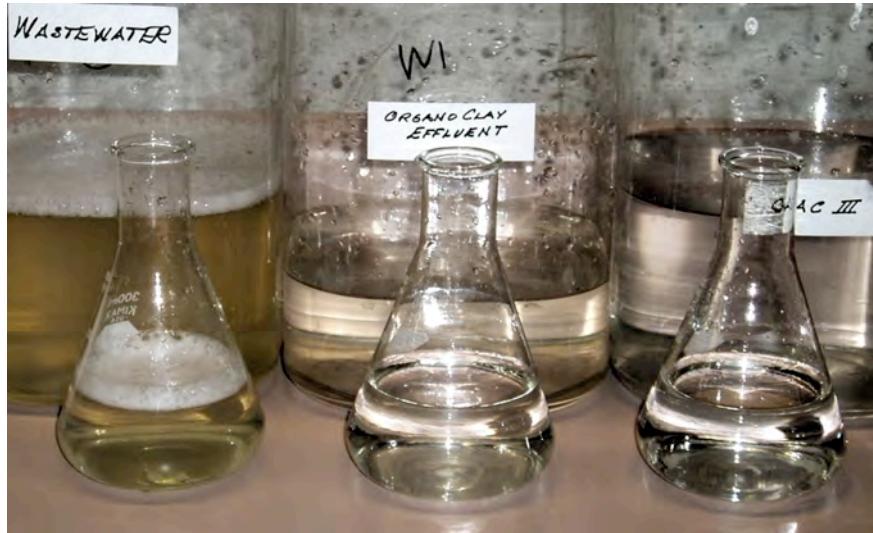
Initial Column Effluents reduced in Foam, Color, Odor and Turbidity
