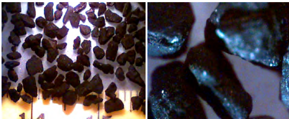
GAC granules (mm scale) and 6x magnification showing rounded edges
