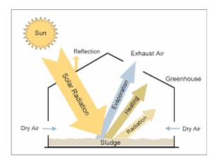
Solar sludge drying beds are not commonplace in the US, but they are currently in service in Europe. Using the energy of the sun in Germany, they operate with a minimal amount of electricity.
