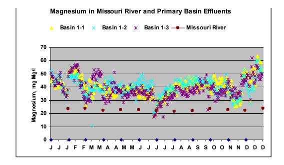
In the absence of supplemental coagulant additions, the concentration of magnesium ion (Mg<sup>2+</sup>, not total magnesium) in the effluent from the primary basin is critical to the subsequent coagulation, flocculation and sedimentation of the lime-treated water in the secondary basin. Data for the year 2000 shows that magnesium in the primary basin effluent varied seasonally. The lowest concentrations were observed in the summer months.
