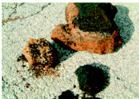
Most of the severely cemented (sandy) material appeared to underlie the anthracite layer. The anthracite also showed evidence of a loose aggregation that could be broken up by hand.
